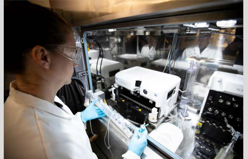
Employee working on a **FASTlab 2** radiochemistry system at GE HealthCare's manufacturing facility in Sweden
